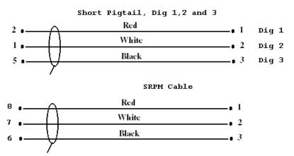
This cable connects to the DIG connector and may have the third RPM (clutch) and the digital channels included.
